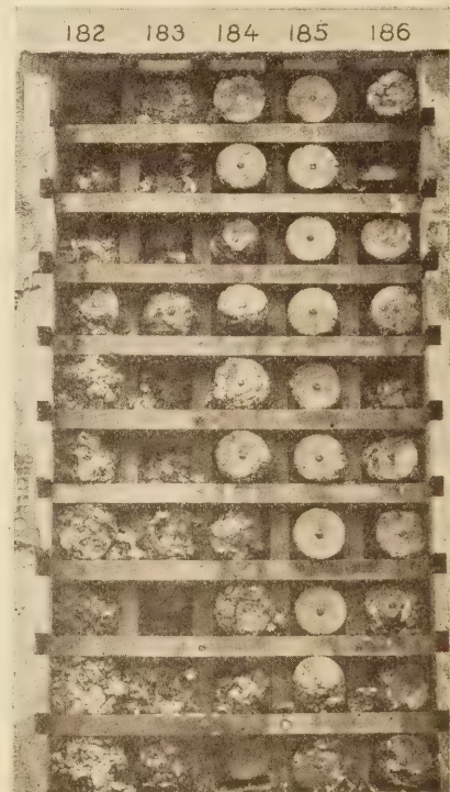
Cylinders with Alkagel "A" admixed in following proportions, after five years in lake: Series 182.—No admixture Series 183.—3 per cent Series 184.—No admixture (cured in water vapor at 155° F., 48 hrs.) Series 185.—3 per cent (cured in water vapor at 155° F., 48 hrs.) Series 186.—3 per cent (cured in water vapor at 100° F., 48 hrs.)
